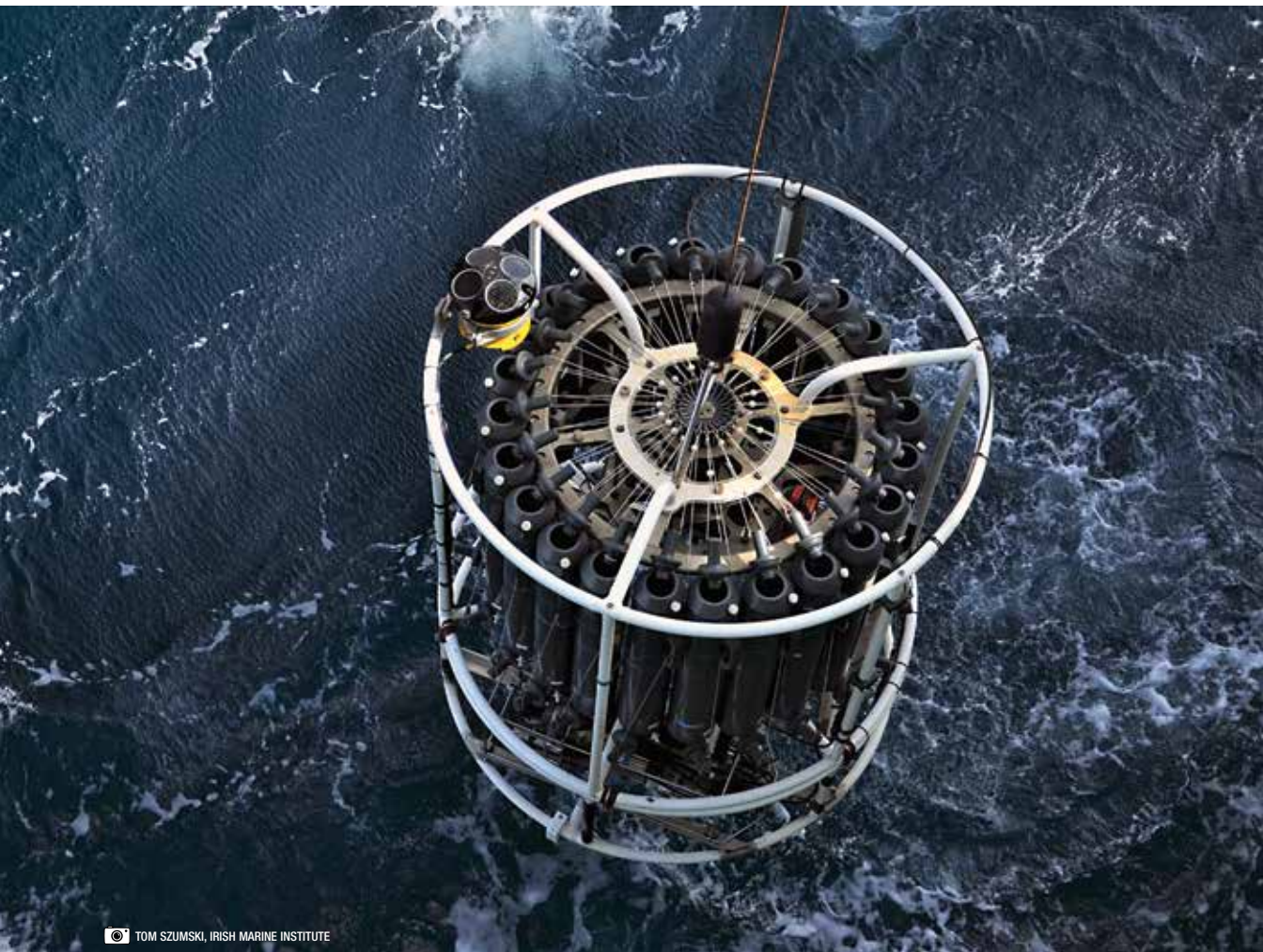
Figure 4: The CTD carousel was lowered to just above the ocean floor and then brought back to the surface in an operation that took up to five hours at the deepest stations of > 4.8 km below the ocean surface.
